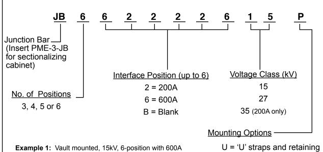
interface on positions 1 and 6, 200A interface on positions 2, 3, 4 and 5, with mounting bracket and parking stand option. Catalog number would be JB662222615P.
