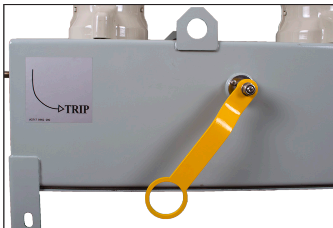
▲ Manual trip handle prohibits electronic closing operation through the control and features mechanical block providing the utmost in safety.
