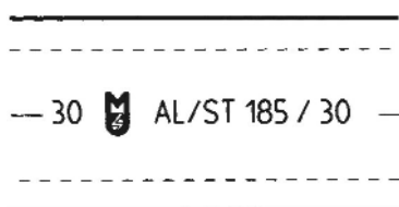
Marking of compression dead end clamps and joints
