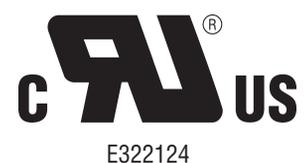
**UL Recognized Component Marks for USA and Canada:** The combined UL signs for the USA and Canada are recognized by the authorities of both countries. All auxiliary relays identified with this mark meet the requirements of both countries.
